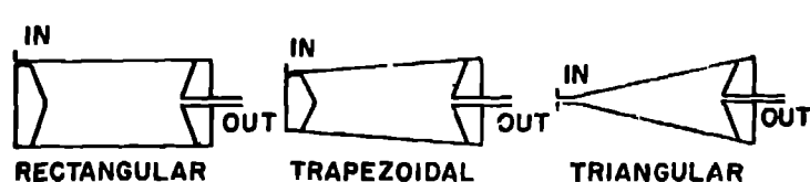
Fig. 7. Variations of the plate generator arising from varying the input plate separation.
